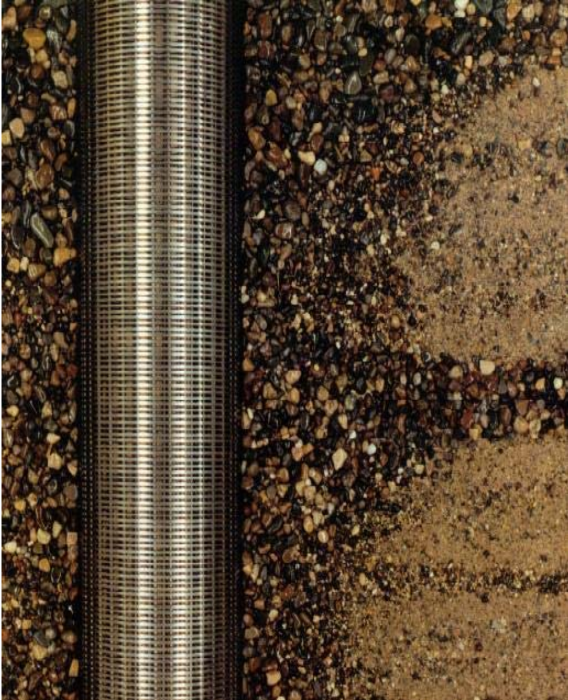
Well Screen Installation after Well Development Illustrating a Typical Natural Gravel Pack (Courtesy Johnson Screens)
